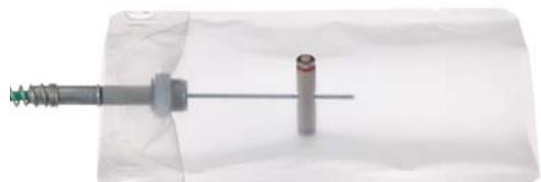
Press the cutting tool either by hand or with a hammer until a hole is cut out.
