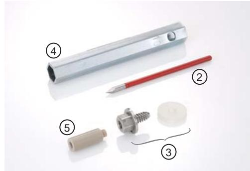
Place the HUJ-C (3) in the TC26 spanner (4) and screw it into the hole.
