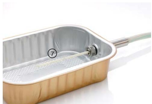
Introduce the multipoint probe into the packing gland.
