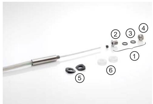
Introduce the bushing (2) mounted with an o-ring or a washer (please see below) into the hole, and place the other o-ring or washer on the bushing from the inside of the container.
